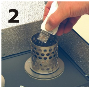
2 Remove Heater Bulb. Note: Use Paper Cover of new Bulb
