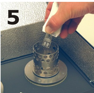
5 Install SMug Heater Bulb
