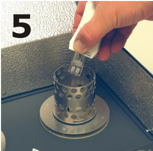
5 Install SMug Heater Bulb
