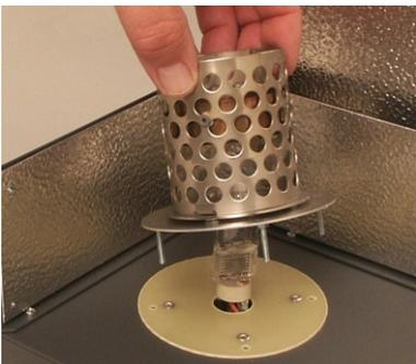
The Heater Cover can be replaced by a different one with different Dimensions for different Products (Future Option).
